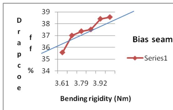
Figure 3: Drape Coefficient Vs Bending Rigidity for Bias Seam
