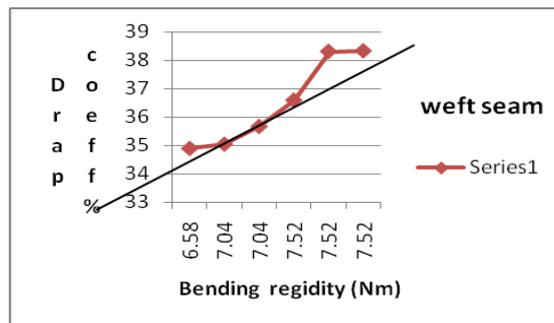
Figure 1: Drape Coefficient Vs Bending Rigidity for Weft Directional Seam
