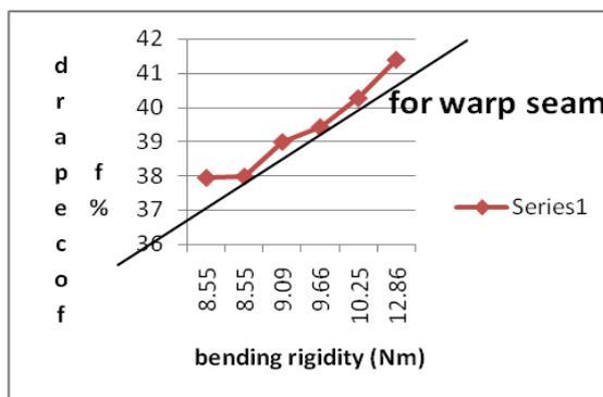
Figure 2: Drape Coefficient Vs Bending Rigidity for Seam in Warp Direction
